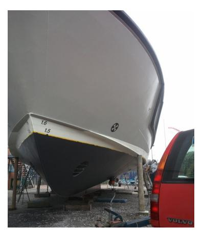
The "pod" for the WASSP transducer is compact and welded to the keel for a very secure and safe mount
