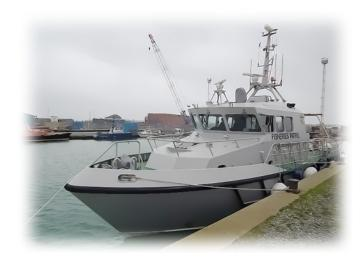
Sussex Inshore Fisheries and Conservation Authority patrol vessel Watchful has recently had a WASSP system installed by oceanDTM. The vessel is capable of collecting good quality data up to a speed of 14 knots.
